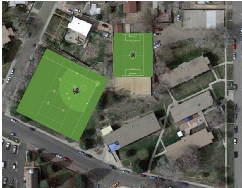
Proposed redesign of grass field and tennis court includes regrading the large field and installing artificial turf; replacing the tennis court with artificial turf for a futsal-sized field. Source: Sprinturf®.
